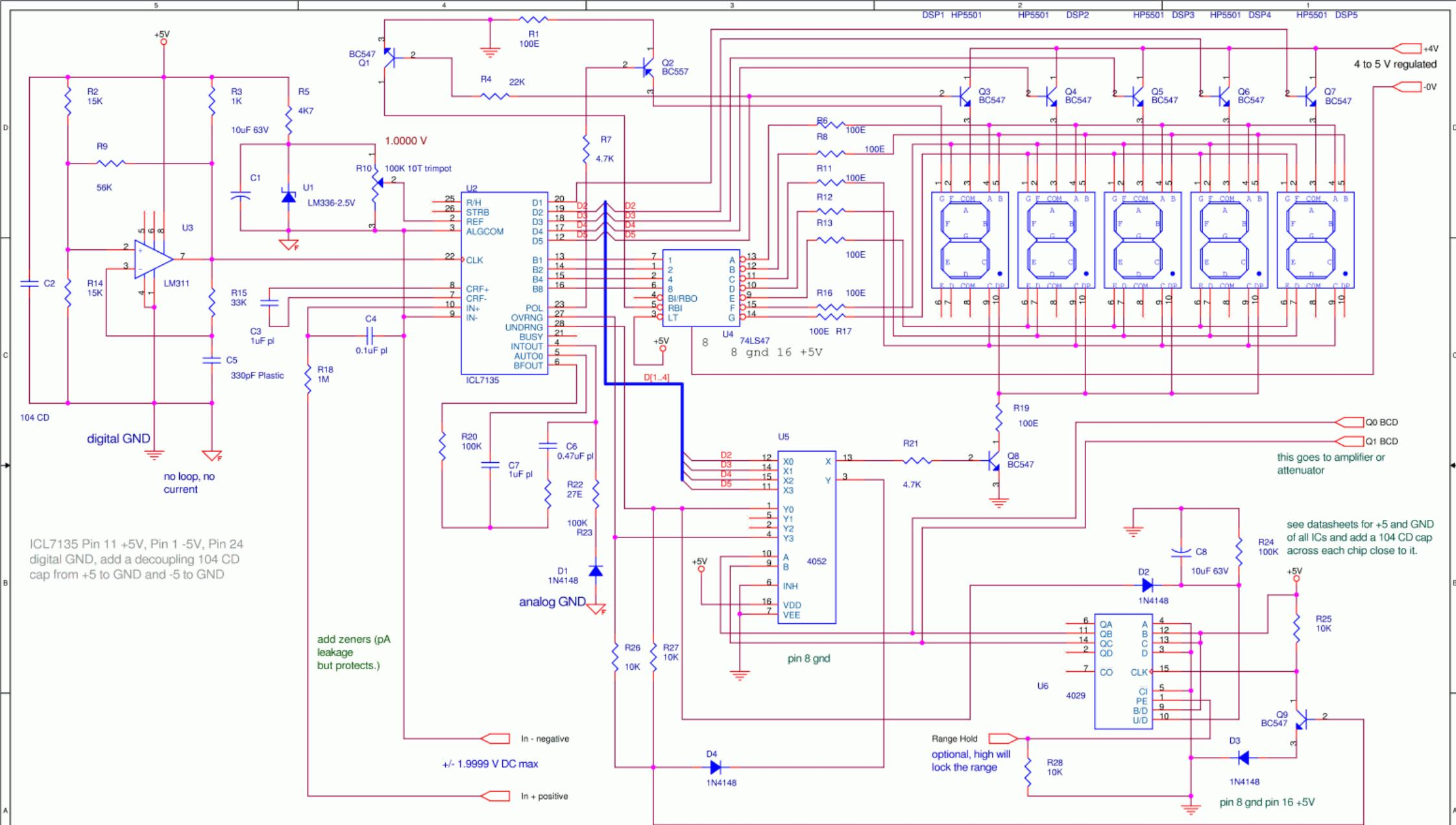
Use Only Low Leakage Multilayer Plastic Capacitors for A-D convertors of Intersil like 7107, 7109, 7106, 7135.
