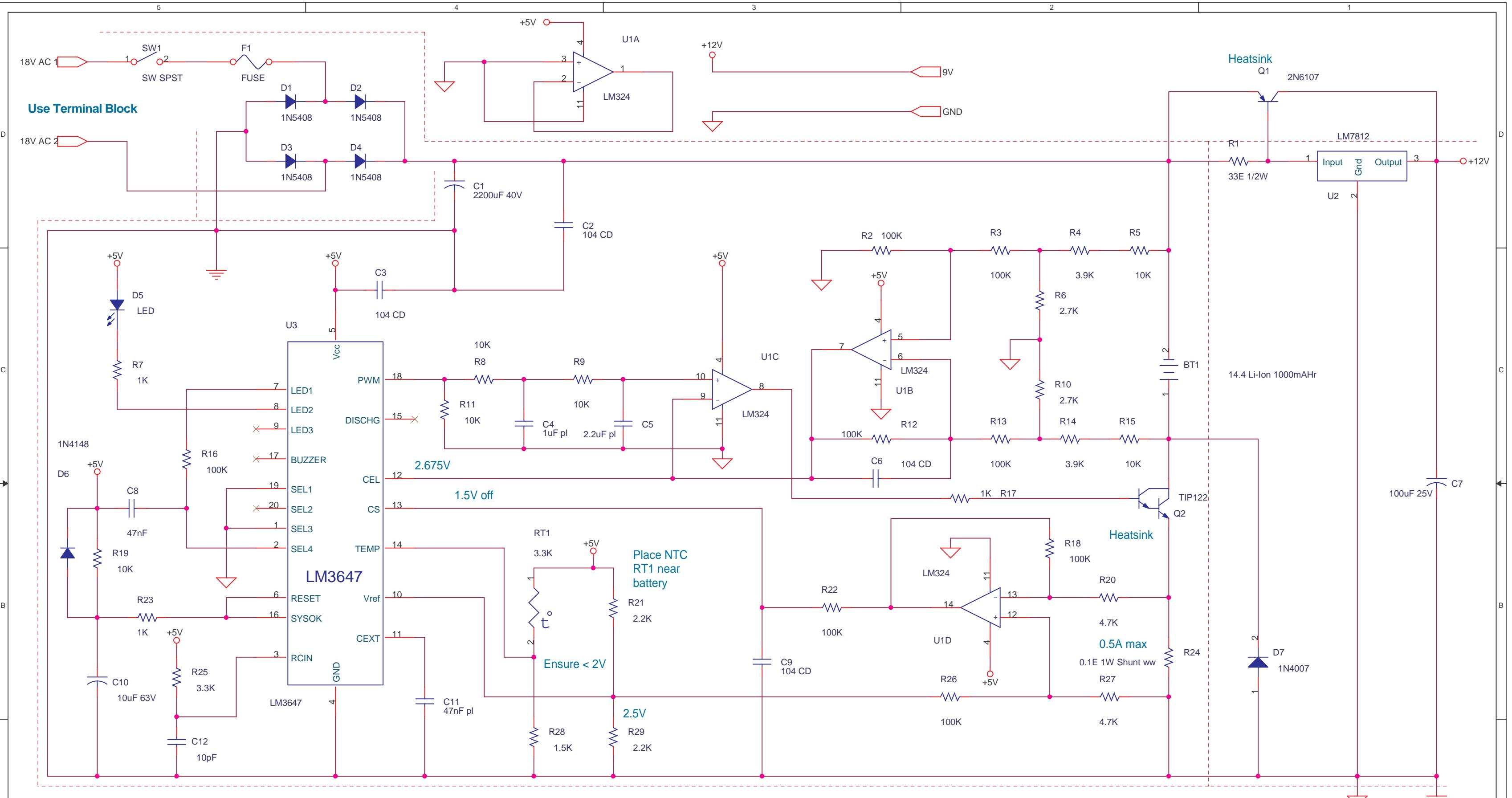
put 104 CD cap for all ICs from positive to negative close to IC, even if omitted in circuit, for opamps on dual supply two caps.
